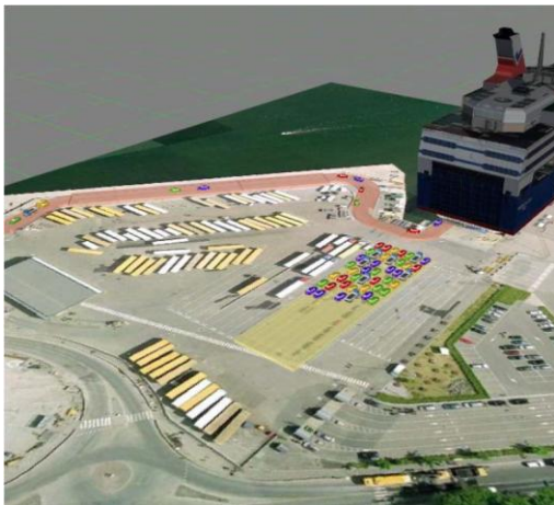
FIGURE 6: 3D VISUALISATION OF THE ABM SIMULATION ENVIRONMENT FOR RO-PAX TERMINAL OPERATIONS [48].
